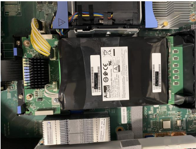
Figure 13 Battery backup unit
