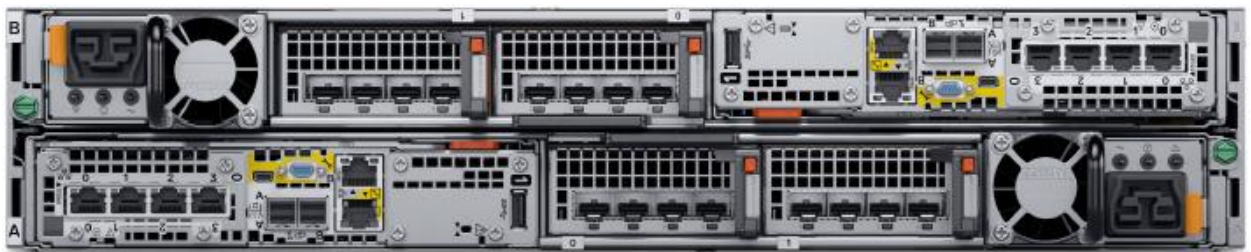
Figure 3 Base enclosure back view
