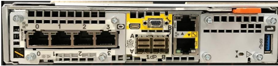
Figure 8 Embedded module with 10/1 GbE BASE-T 4-port card
