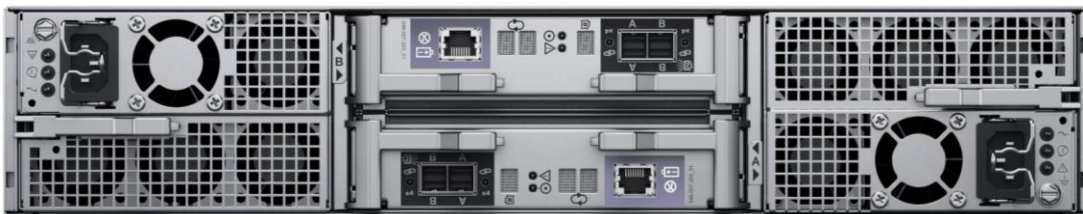
Figure 19 25-drive 2.5-inch 2U expansion enclosure (back)
