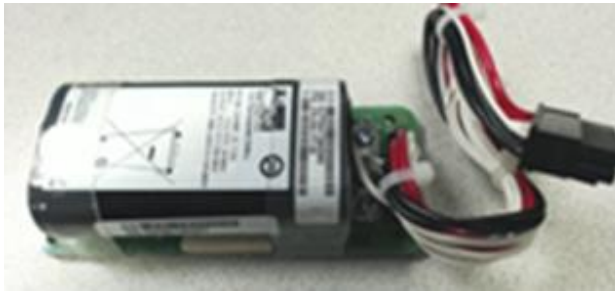
Figure 6 Battery backup unit
