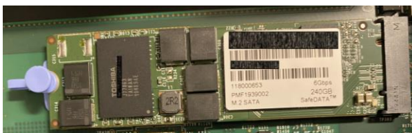
Figure 11 Internal M.2 boot module
