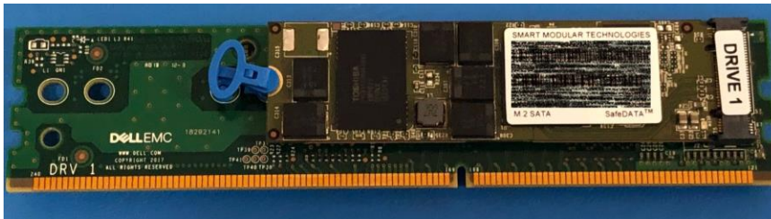
Figure 4 Internal M.2 boot module
