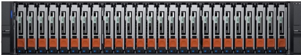
Figure 18 25-drive 2.5-inch 2U expansion enclosure (front)
